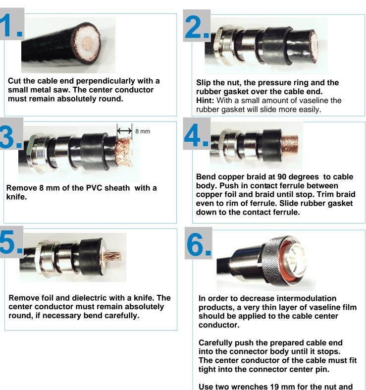
Use two wrenches 19 mm for the nut and 24 mm for the connector body, tighten the nut until there is a small visible gap between the nut and the connector housing. Be careful not to overtighten the nut!!
