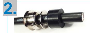
Slip the nut, the pressure ring and the rubber gasket over the cable end. Hint: With a small amount of vaseline the rubber gasket will slide more easily.
