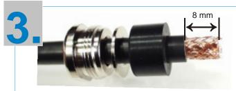
Remove 8 mm of the PVC sheath from the end of the cable with a knife.
