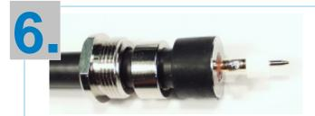
Slide center pin (Pin 1, 2,8mm  $\varnothing$ )on center conductor and solder carefully. Then attach teflon isolator.
