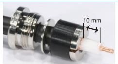
Remove foil with a knife. Trim the dielectric to a length of 10 mm.
