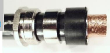
Bend copper braid at 90 degrees to cable body. Push in contact ferrule between copper foil and braid until stop. Trim braid even to rim of ferrule. Slide rubber gasket down to the contact ferrule.
