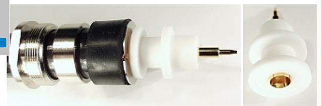
Push center pin in teflon isolator. Then put center pin cautiously on center conductor. **Hint:** Before attaching the center pin a very thin vaseline film may be applied to the center conductor. This improves the intermodulation attenuation and prevents corrosion.
