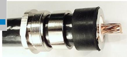
Remove foil and dielectric with a knife. The center conductor must remain absolutely round, if necessary bend carefully.
