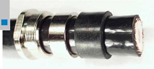
Slip the nut, the pressure ring and the rubber gasket over the cable end. **Hint:** With a small amount of vaseline the rubber gasket will slide more easily.
