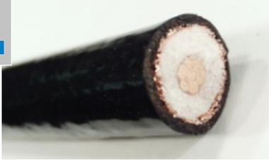
Cut the cable end perpendicularly with a small metal saw. The center conductor must remain absolutely round.
