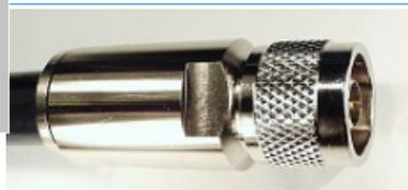
Slide the prepared cable end into the connector housing until stop. Tighten smoothly with two wrenches 19 mm, so that there is still a small gap visible between the nut and the connector housing.
