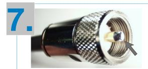
Solder the center conductor carefully to the connector tip.
