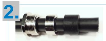
Slip the nut, the pressure ring and the rubber gasket over the cable end. Hint: With a small amount of vaseline the rubber gasket will slide more easily.
